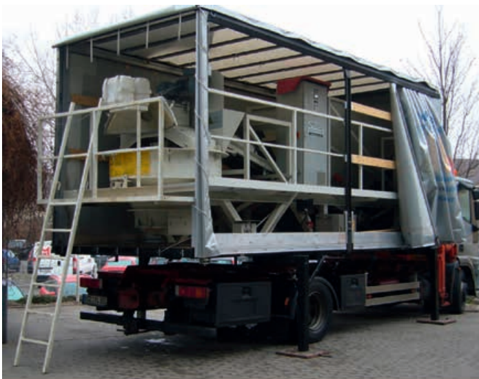
Mobile mixing plant for terrazzo
