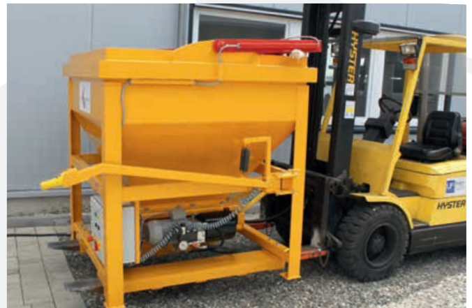
Concrete bucket for SCC, UHPC with hydraulic slide and screw-type agitator
