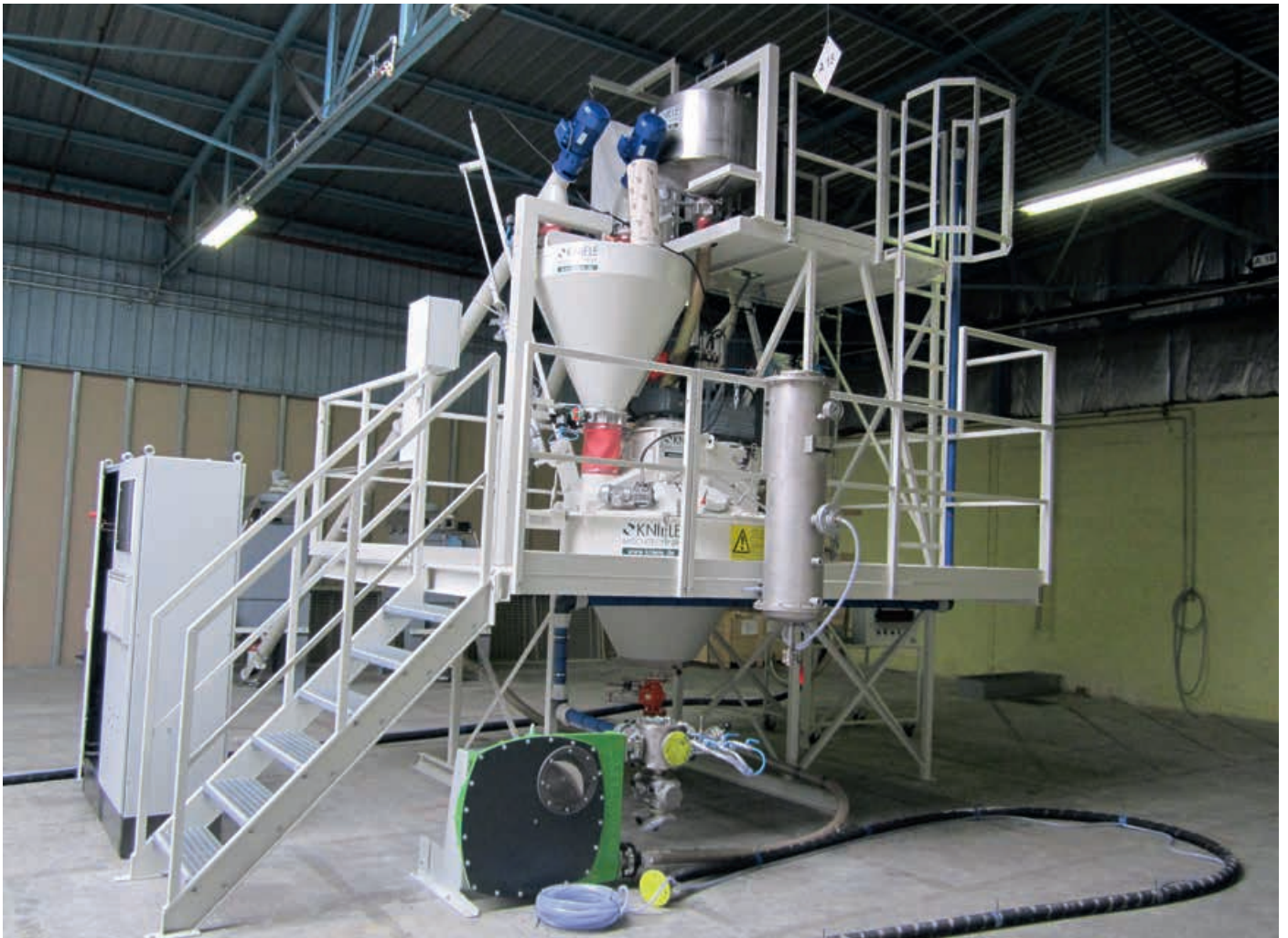
Mixing plant for suspensions with concrete pump and pigging station to clean the hoses (UHPC)
