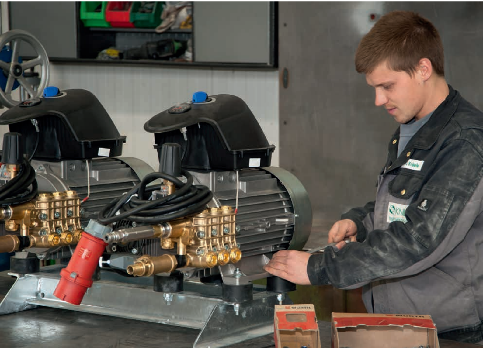
Assembly of the high pressure pumps for the automatic mixer cleaning
