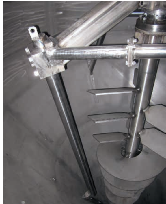
Agitator, Cone Mixer KKM in stainless steel
